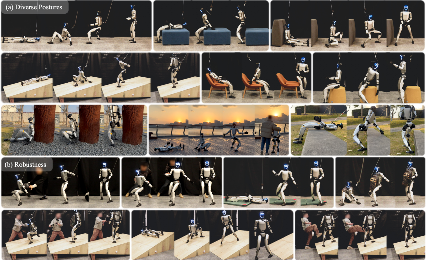
Fig. 1: Overview. (a) Our proposed framework HoST enables the humanoid robot to learn standing-up control via reinforcement learning without prior data, where the robot can successfully stand up across diverse postures in both laboratory and outdoor environments. (b) HoST also demonstrates strong robustness to many environmental disturbances, including external forces, stumbling blocks, 12kg payload, and challenging initial postures.
